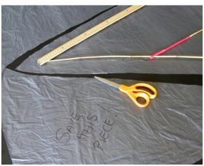
Step 11 Re-align the vertical and leading edge spars with the lines you drew on the plastic. Fold the excess plastic over the leading edge spars and tape the plastic over the frame using four 40 cm lengths of tape (two for each side). Don't tape over any of the intersections where two spars overlap.
