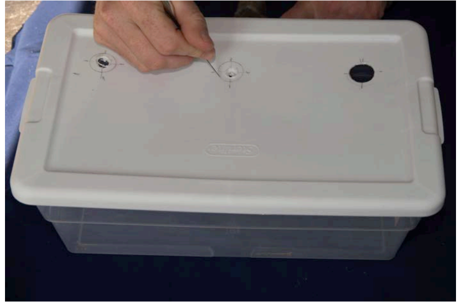
New box tops are fairly flimsy, which in this case is a good thing. It makes them easier to cut with a hobby knife. Carefully cut out the nickel tracings using the hobby knife. (A large hot-glue gun can also be used to melt holes of the desired size).
