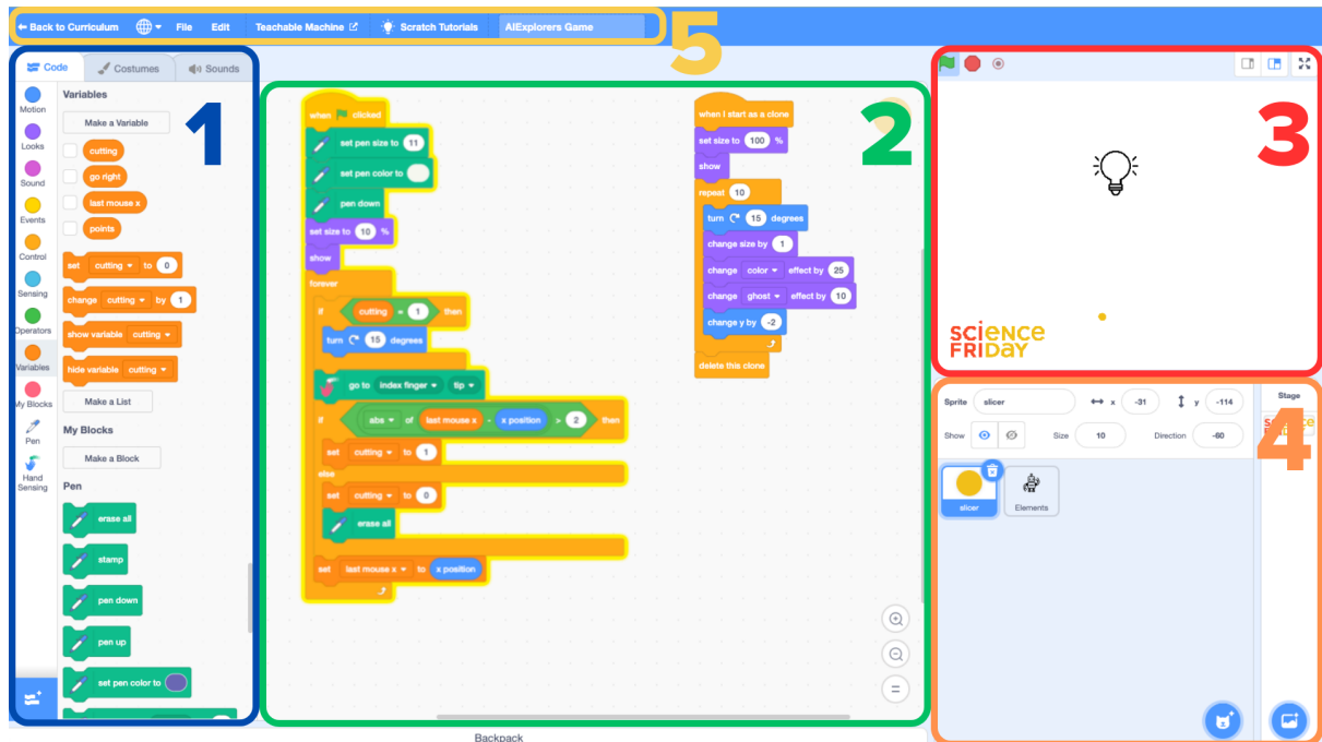
(1) The tabs for code blocks, costumes, and sounds. (2) The Code Area. (3) Stage. (4) Sprite Pane. (5) Toolbar. Created in Canva by Science Friday using a Scratch screen capture.
