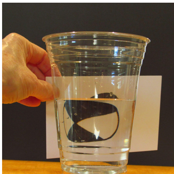
The Secchi disk can be seen easily, showing that the water is clear. Credit: Kathy Ceceri
