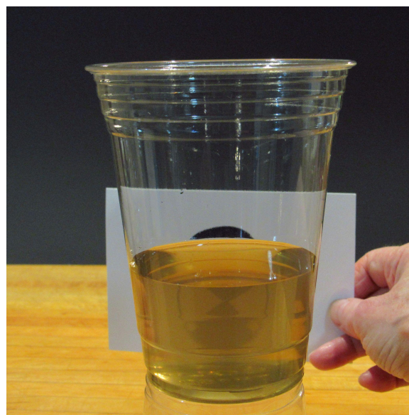
The Secchi disk cannot be seen, indicating this water is contaminated. Credit: Kathy Ceceri
